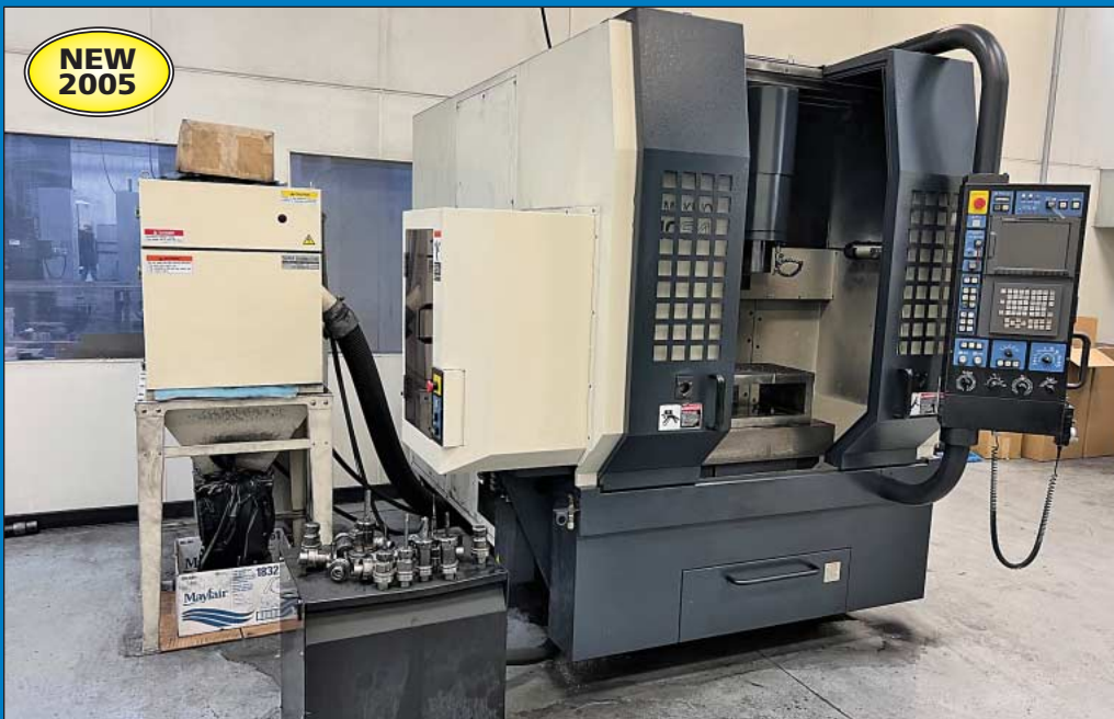
Makino Model SNC64 CNC Graphite VMC (2005)
