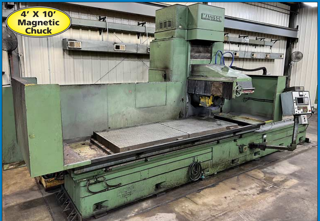
4' X 10' Mattison CNC Hydraulic Surface Grinder w/ Fanuc Powermate Control
